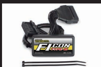
FI CON TYPE-e (injection controller)
