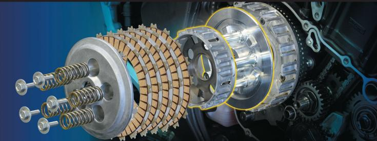
While the slipper clutch downshifting rapidly, the clutch will be slipped for relieving the back torque. It is possible to reduce the burden on the transmission, hopping of rear tire by the engine brake.
