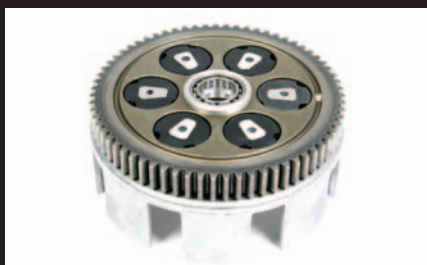
inner structure of primary driven gear (Rubber damper built-in)
