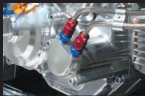
Image after installation : Oil cooler unit
