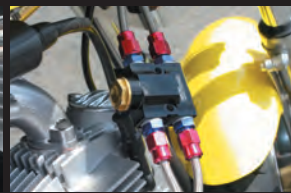
Image after installation : In-line thermostat unit
