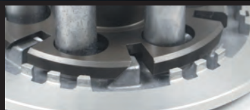
at operation of slipper mechanism
