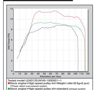
Stock engine+standard pulley+standard exhaust system
