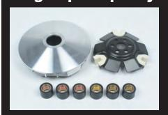
It is a high-speed pulley kit suitable for stock engine, in stock exhaust system. \*\*At the replacement of the high-speed pulley, universal holder is required.
