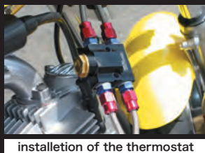
installation of the thermostat
