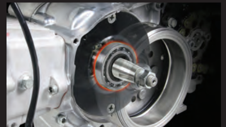
Installing a ball bearing in the support plate
