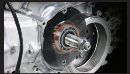
Installing a ball bearing in the support plate
