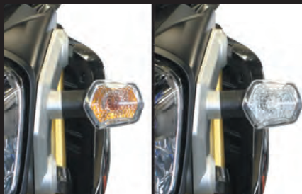
MSX125 / Unlit (Left : stock bulb Right : LED bulb)
