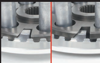
Normal condition (left) and Slipper clutch actuation condition (right)
