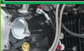
Change the oil line of the cylinder head to pass through oil filter.
