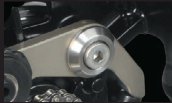
Adopted exclusive mount adopter to hold the tensioner arm from vibrations.
