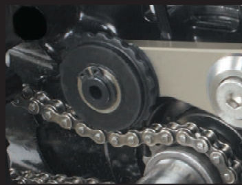
By adopting the sprocket gear tooth, it improves followability to the cam chain.
