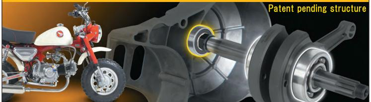
The flywheel is very heavy and attached to the end of the crankshaft, which burdens such as twisting and deflection are applied to the shaft. Along with the high rotation and high output of the engine, this burden increases and it becomes a harsh state.
