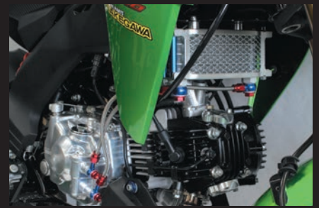
Our oil cooler can be installed in the shroud bracket
