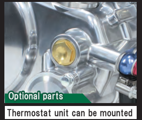
Thermostat unit can be mounted
