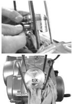
Fix the supplied piston pin circlip. Arrange the position of the ring-end gap of the piston pin circlip not to be on the notch.
