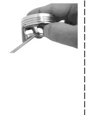
With reference to the figure below, fix piston rings with a letter N facing upward.
