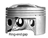
Air-blow the piston rings and the piston pin, and check for their jamming any foreign material.
