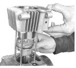
Compressing the piston rings, install the cylider with care not to get the ring-end gaps out of alignment.
