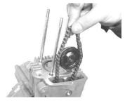
Temporarily tighten the cam chain guide roller and cylinder side bolt for the moment.
