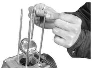
Fix a supplied cylinder gasket into the cylinder base of the crankcase.
