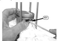
Remove the waste cloth used to clog the holes.
