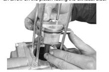
Plug the sleeve hole and the cam chain hole on the crankcase with a clean cloth, and fix a piston pin circlip.
