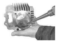
Fit the aluminum cylinder into the stud bolt.
