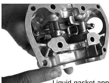
Liquid gasket application
