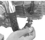
Tighten two nuts on the exhaust pipe loosely for now Tightening torque: 10 N⋅m (1.0 kgf⋅m) Tool to use
