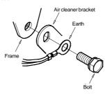
Tools to use: 10mm socket & medium-sized extension bar Tightening torque:10 N· m (1.0 kgf· m)
