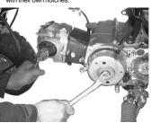
Remove two hex bolts on the cam sprocket by turning counterclockwise while stop rotating the flywheel. Tools to use:
