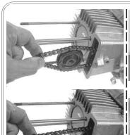
Press in the guide roller to align the center of the guide roller and the guide-roller bolt hole.
