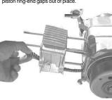
Once the piston has been placed inside the cylinder, pass the cam chain through the cylinder, and fix the cylinder into the crankcase.
