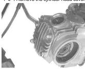
Remove four nuts holding the cylinder head cover by turning counterclockwise in a crisscross pattern. Remove four washers beneath the nuts.
