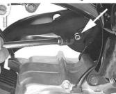
Remove the nut fixed at the reverse side of the exhau system by turning counterclockwise
