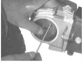
Gently pry the cam sprocket loose to remove from the camshaft with a small-sized slotted screwdriver.
