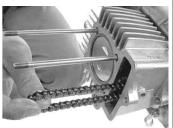
Fix the guide roller while pulling the cam chain.
