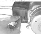
Remove the loosened guide roller bolt and cylinder side bolt by turning them counterclockwise.
