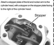
Apply molybdenum to the stock rocker arm shaft. Then align the holes of rocker arm and stpper plate and
