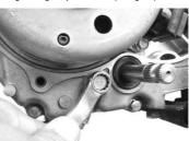
Install the hex bolt which was next to the change ped and was just removed.
