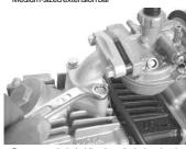
Remove two bolts holding the cylinder head and inlet pipe
