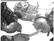
Tighten up two cam sprocket bolts while stop rotating the flywheel.
