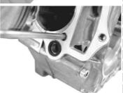
Install the cylinder gaskets and rubber seal
