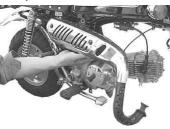
Installing the exhaust system, route the tail pipe insid the rear shock absorber first, and then run the flange close to the exhaust outlet of the cylinder head.
