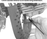
Remove two collars of the flange and then remove the exhaust system from the motorcycle by pulling it outwards
