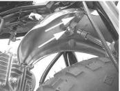
Remove two hex bolts on the reverse side of the front fender by turning them counterclockwise. Tools to use:
