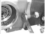
Remove the cylinder-head side bolt holding the cylinder head and cylinder, by turning it counterclockwise.
