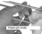
Remove one of the piston pin circlips with a screwdriver tip.
