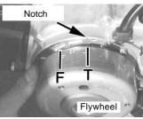
Turn the flywheel counterclockwise so a "T" mark on the flywheel and "O" mark on the cam sprocket align with their own notches
