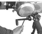
Remove the hex bolt on the shift pedal, and turn the shift pedal counterclockwise to remove it. Tool to use
