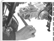
Tighten the head nuts in a crisscross pattern in two
