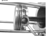
You can rather easily install the piston pin circlip by pressing it with a screwdriver, but taking care not to damage the piston with the screwdriver. Do the work carefully as, in some cases, the circlip comes off flying while you are pressing it inside. So, wear protective eyeglasses for your eyes.
