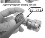
Set the cam shaft on the cylinder head of the kit
