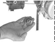
While removing the cylinder, the cam chain guide roller will come out, which please remove.
