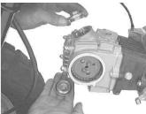
Remove two tappet caps by turning counterclockwise.
