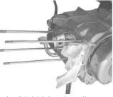
Plug the cylinder hole in the crankcase with a waste cloth to avoid entering any unwanted parts into the cylinder hole and cam chain.
