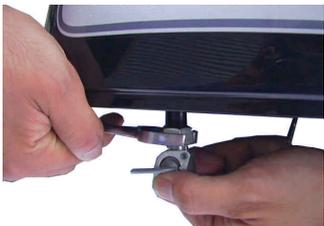
Insert a fuel tube and fasten it with a tube clip. Open the fuel cock and check for gas leaks. (Do not leave the cock open for long time.)
