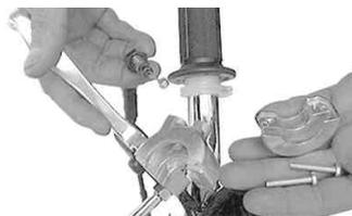
Fix an ground wire to the frame with an air-cleaner-mounting bolt.
