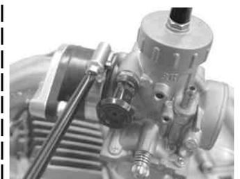
Attach an air filter, which please fix by tightening a band.
