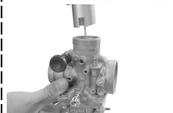
Fit the carburetor into the insulator, and fasten the carburetor with a clamp band.
