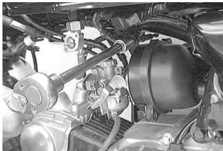
Remove the throttle valve from the carburetor, and separate the throttle valve from the throttle cable. Then pull out the top cover from the throttle cable.
