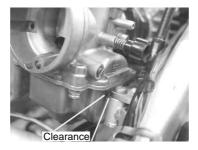
Tighten an insulator band to hold the carburetor firmly.
