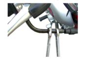
8 . Connect the fuel tube, open the fuel cock, and check each section for oil leaks.
