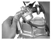
Unscrew a screw on the throttle housing to take out the throttle cables. And change the throttle cables.
