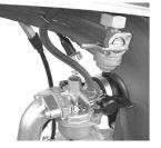
Loosen a band on the air-cleaner connecting tube, and pull out an inlet-pipe holding bolt, and remove the carburetor with the inlet pipe and all.
