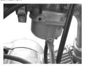
2 . Remove the fuel tube and throttle valve from the carburetor, and separate the throttle valve from the throttle cable.
