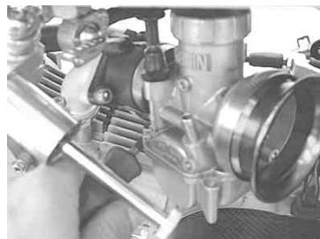
Adjust the free play at the throttle grip to be about 5 mm and check that the throttle has free play even when a steering handle is turned all the way to the right or to the left. Snap the throttle a few times to make sure that the throttle moves smoothly without sticking and that the throttle valve is fully open.
