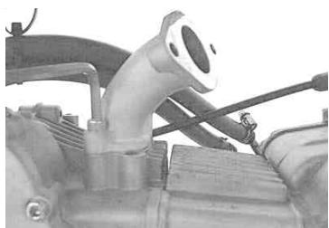
Install an insulator onto the inlet pipe with two M6x15 socket cap screws.
