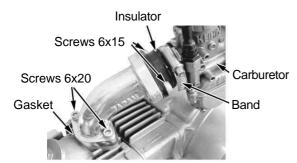
Place the carburetoe into the insulator, and tighten the band to secure it.
