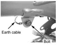
Unscrew a bolt on the storage tank, and pull out a breather hose from the crankcase.
