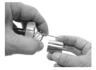
Attach the throttle valve to the carburetor, aligning the notch with the throttle stop screw.
