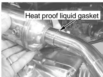
It is advisable to apply heat-resistant liquid gasket to the inserting portion.
