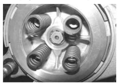
7 . Fix the 6x22 hex flange bolt on the clutch pressure plate and tighten them with hand properly, with the bearing of the clutch lifter plate facing outside.
