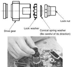
2 . Install the clutch bearing seat into the transmission mainshaft. (Set the bearing seat so its folded portion fits well with the crankcase so as to prevent it from rotating.)
