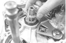
3 . Apply engine oil to the ball bearing of the primary driven gear COMP., and then the grease to the oil seal. And insert the primary driven gear COMP. into the mainshaft.
