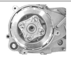
8 Install the dry clutch cover referring to the instruction manual.
