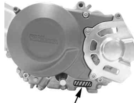
Engine No. stamped here. 4SMP-00***
