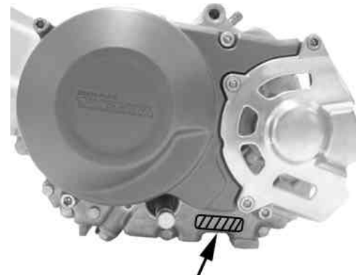
Engine No. stamped here. CSMP-00***
