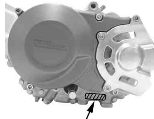
Engine No. stamped here. 4SMP-10***
