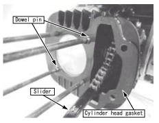
O Place the cam chain through the cylinder head and install the cylinder head.
