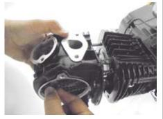
O Install x4 washers, head nuts and x2 cylinder head side bolts.
