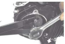
O Remove the tensioner rod oil filler bolt.
