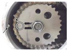
O Fix the cam sprocket with a universal holder, remove the cam sprocket bolt/ washer, and remove the cam sprocket.
