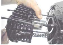
O Align the guide roller with the cylinder mounting hole and temporarily tighten the guide roller bolt/new sealing washer.
