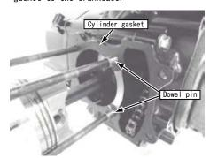
O Apply engine oil to the piston ring and let it blend in Apply engine oil after cleaning the inner circumference of the cylinder.
