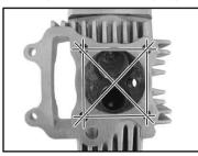
Service limit: If the distortion is over 0.05 mm, replace the cylinder head.
