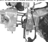
Attach the cylinder head plate and tighten the head nuts evenly.
