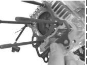
Install the cylinder head, fitting the cam chain and stud bolts in place.
