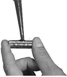
Install the piston to the connecting rod with the IN mark on the piston facing the intake side.
