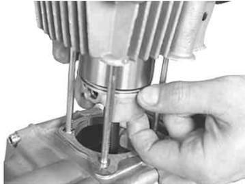
Place the cam chain guide roller inside the cam chains, as shown in the figure below.
