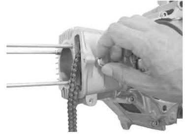
Install the cylinder head with reference to its instruction manual.
