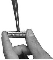
Install the piston to the connecting rod with the IN mark on the piston facing the intake side.
