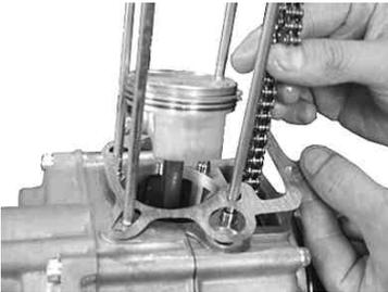
Fix a supplied new rubber packing (black) onto the oil-return hole on the cylinder base of the crankcase.
