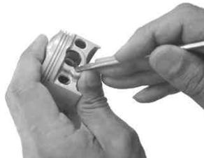
Attach the piston pin circlip so the ring end gap does not meet with the notch on the piston pin hole, and it should be either on the top or at the bottom of the hole as illustrated in the figure below.
