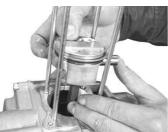
Plug the sleeve hole and the cam chain hole on the crankcase with a clean cloth, and fix a piston pin circlip.
