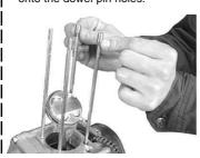
Fix a cylinder gasket of the kit into the cylinder base of the crankcase.
