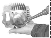
Insert the aluminum cylinder into the stud bolts.
