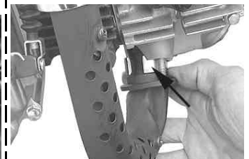
Detach two collars of the flange and then detach the muffler from the motorcycle by pulling it outwards.
