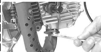
Remove two nuts on the exhaust pipe by turning them counterclockwise. Tool to use Open-end wrench, 10 mm
