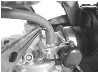
Shift the tube clip to disconnect the fuel tube of the carburetor.
