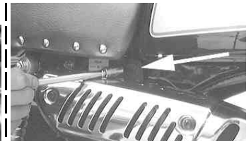
Remove the hex nut securing the muffler by turning it counterclockwise.
