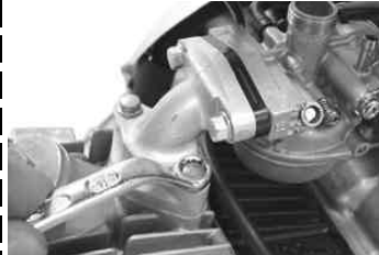
Unfasten two bolts attaching an inlet pipe to the cylinder head to remove the inlet pipe, carburetor, and air cleaner. Tool to use Offset box wrench, 8 mm
