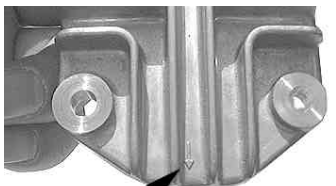
Attach the cylinder-head-cover gasket and head cover.
