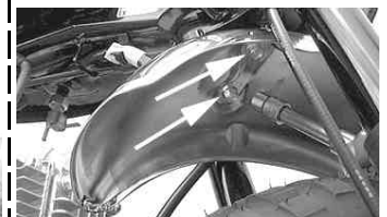
Remove two hex bolts on the reverse side of the front fender by turning them counterclockwise.
