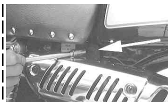
Remove the hex nut securing the muffler by turning it counterclockwise.
