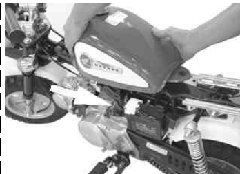
Pull the fuel tank backward to demount it.
