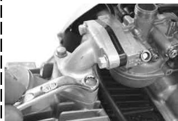
Unfasten a bolt on the air-cleaner stay. Tool to use Socket, 10 mm Extension (short)
