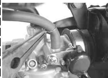
Remove the fuel cock and install the one in the kit. Tool to use Open-end wrench, 19 mm
