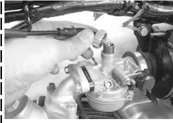
Remove a top cap and pull out a throttle valve, from the carburetor.
