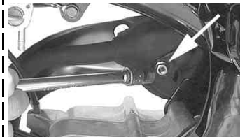
Remove the nut, fastened on the rear side of the muffler, by turning it counterclockwise.
