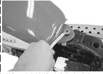
Unfasten the bolt holding the fuel tank to the frame. Tool to use Offset box wrench, 10 mm
