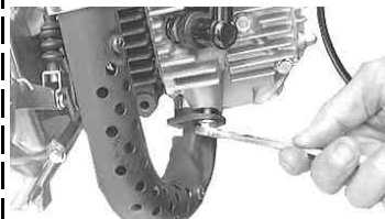
Remove two nuts on the exhaust pipe by turning them counterclockwise. Tool to use Open-end wrench, 10 mm
