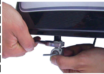
Remove the fuel cock and install the one in the kit. Tool to use Open-end wrench, 19 mm
