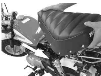
Pull the seat backward to demount it.
