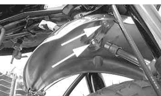
Remove two hex bolts on the reverse side of the front fender by turning them counterclockwise.
