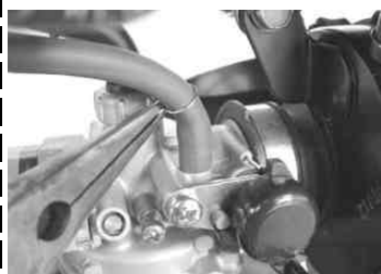
Remove the fuel cock and install the one in the kit. Tool to use Open-end wrench, 19 mm
