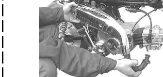
Fix the earth wire to the frame with a bolt on the air-cleaner stay. Tool to use Socket, 10 mm Extension (short)
