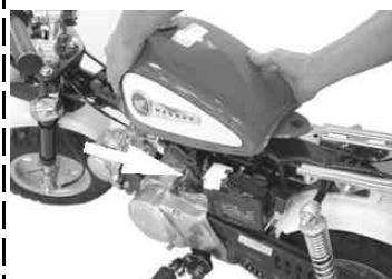
Dismantle a fuel tank by pulling it backwards.
