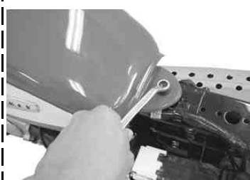
Unfasten a bolt holding the fuel tank to the frame. Tool to use Offset box wrench, 10 mm
