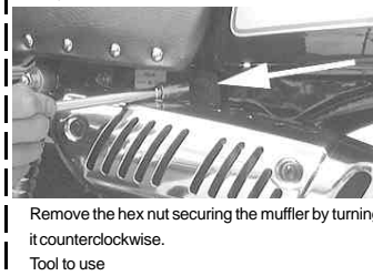
Remove the hex nut securing the muffler by turning it counterclockwise. Tool to use Socket, 12 mm Extension (medium)
