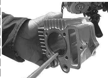
Apply engine oil onto the inside of the supplied cylinder and spread the oil evenly with fingers.
