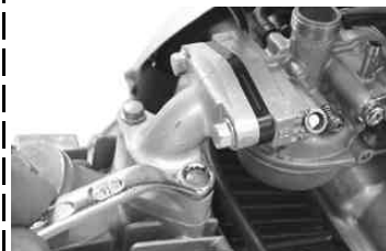
Unfasten a bolt on the air-cleaner stay. Tool to use Socket, 10 mm Extension (short)
