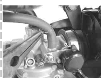
Remove the fuel cock and install the one in the kit. Tool to use Open-end wrench, 19 mm
