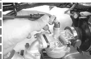
Remove a top cap and pull out a throttle valve, from the carburetor.
