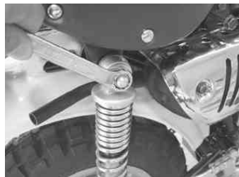
Loosen a nut under the seat to unfasten a bolt. Tool to use Socket, 12 mm Extension (short) Offset box wrench, 10 mm
