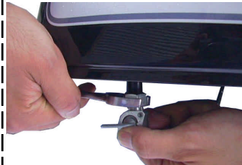
Remove the fuel cock and install the one in the kit. Tool to use Open-end wrench, 19 mm
