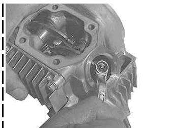
Detach tappet nuts and bolts on the rocker arm assembled into the cylinder head. At the time the tappet nuts are loosened, detach the tappet bolts and nuts together.
