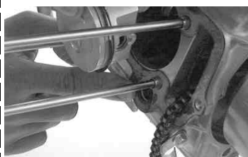
Install the cylinder gaskets and rubber packing.
