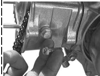
Install a cylinder side bolt. (Tighten it only finger tight at this point.)
