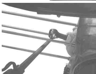
Apply engine oil to the piston pin and con'rod, and install the piston pin.
