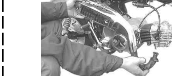
Fix the earth wire to the frame with a bolt on the air-cleaner stay. Tool to use Socket, 10 mm Extension (short)
