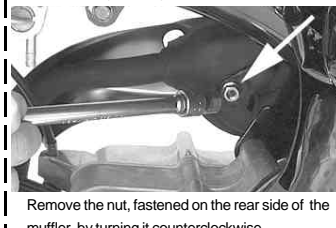
Remove the hex nut securing the muffler by turning it counterclockwise. Tool to use Socket, 12 mm Extension (medium)
