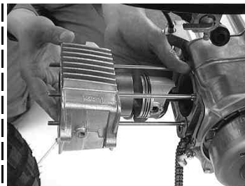
Pressing the tire, install the cylinder.
