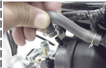
In the case of a motorcycle with a frame No. of AB27- pull out the hose on a storage tank hose.
