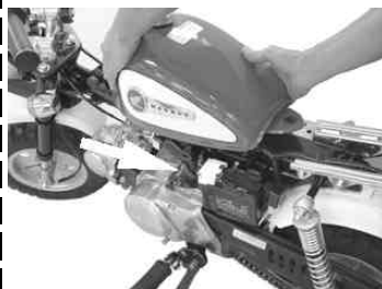
Pull the fuel tank backward to remove it.
