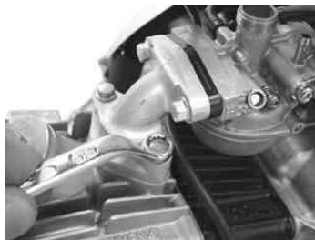
Unfasten a bolt on the air-cleaner stay. Tool to use Socket, 10 mm Extension (short)
