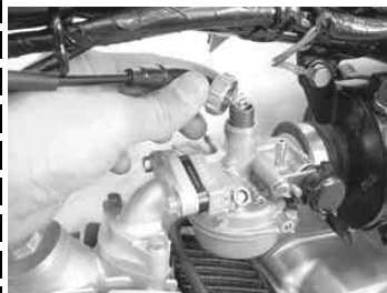
Remove a top cap and pull out a throttle valve, from the carburetor.
