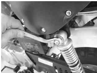
Loosen two nuts on the rear shock absorber. Tool to use Offset box wrench, 14 mm
