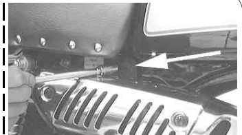
Remove the hex nut securing the muffler by turning it counterclockwise.
