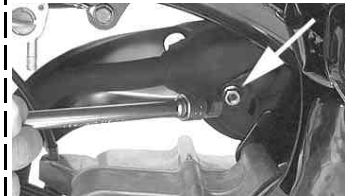
Remove the nut, fastened on the rear side of the muffler, by turning it counterclockwise.
