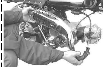
Clamp Wire harness Move the wire harness so it sits under the frame.
