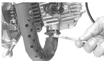
Remove two nuts on the exhaust pipe by turning them counterclockwise. Tool to use Open-end wrench, 10 mm
