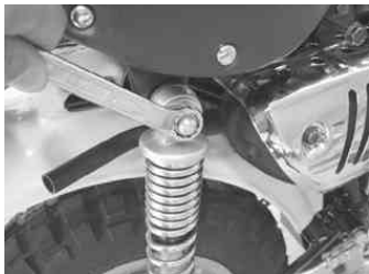
Loosen a nut under the seat to remove a bolt. Tool to use Socket, 12 mm Extension (short) Offset box wrench, 10 mm
