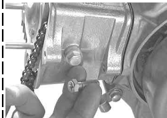
Install the cylinder side bolt. (Temporarily tighten it as tight as possible by hand.)
