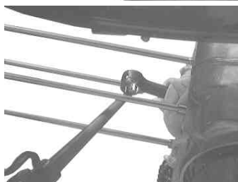
Apply engine oil to the piston pin and the connecting rod, and install the piston pin.
