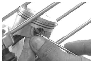
You can rather easily install it by pressing it into the piston with a screwdriver, but taking care not to damage the piston with a screwdriver. Do the job carefully as, in some cases, the circlip comes off flying while you press it inside. So, wear protective eyeglasses for your eye protection. Take away the waste cloth.
