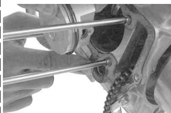
Fix the cylinder base gasket and a black rubber packing.
