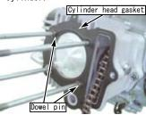
In the case of a monkey, push the tire rubber by hand (to make space) and install the cylinder head through the stud bolt.
