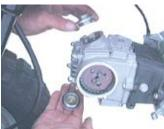
◇Turn the flywheel counterclockwise so a "T" mark on the flywheel and "O" mark on the cam sprocket align with their own notches.
