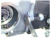
Loosen a guide roller bolt on the cylinder and a side bolt between the cylinder and crankcase.
