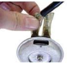
IInstall the fuel cock with two screws.
