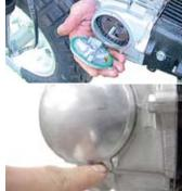
♦ Tighten the sealing washer and the hexagon bolt(arrow) on the right side of the cylinder head.
