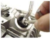
♠After adjusting the tappet, turn the flywheel counterclockwise twice by hand, and then, align "T" and "O" marks each other.
