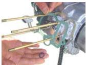
Cut off the gasket, if any, squeezing out into the section pointed by a finger as shown in the picture.
