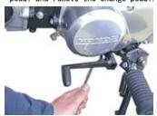
Remove three bolts which are holding a crankcase left-side cover.
