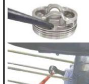
the piston head faces downward, or to the exhaust side.
