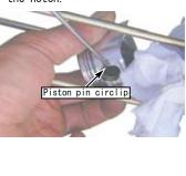
Remove the piston pin in the direction where the piston circlip is not attached. You can easily remove the piston pin by pressing it with a flat tip screwdriver from the direction where a piston pin circlip is
