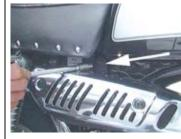
◇ Turn a nut, fixed at the reverse side of the exhaust system, counterclockwise to remove it.
