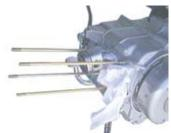
Remove one of the two piston pin circlips. You can remove it by prising it open with a screwdriver tip being placed on the notch
