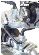
Disconnect the hose on the storage tank in the case of bikes with frame Nos AB27-.
