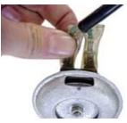
IInstall the fuel cock with two screws
