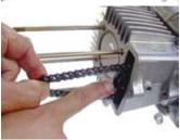
Install the guide roller bolt. (Fasten it only finger tight for now at this point.)
