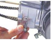
♦ Attach the cylinder side bolt. (Fasten it only finger tight for now at this point.)
