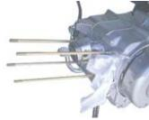
Remove one of the two piston pin circlips. You can remove it by prising it open with a screwdriver tip being placed on the notch.
