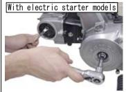
Install the hex bolt which was next to the change pedal and was just removed.
