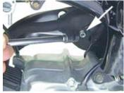
♦ At this point, loosely install a hex bolt which holds the exhaust system
