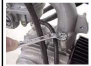
♦ Connect wires to the horn.
