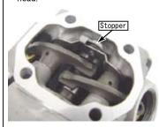
Apply molybdenum to the stock rocker arm shaft. Then align the holes of rocker arm and stpper plate and fix the rocker arm shaft.
