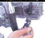
Attach a nut on the reverse side of the muffler loosely for now.
