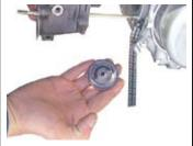
Once the piston has come out, pull out the cylinder forward, holding the tire with a hand.
