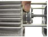
Once the piston has been placed inside the cylinder, pass the cam chain through the cylinder, and fix the cylinder into the crankcase.
