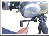
♦ Turn three bolts counterclockwise which hold the generator cover.
