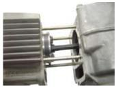
⇒ Fit in the cylinder, by installing the piston rings one by one with fingers, being careful not to move the piston ring-end gaps out of place.
