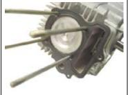
Install the cylinder head while fitting the cam chain and stud bolts in place.
