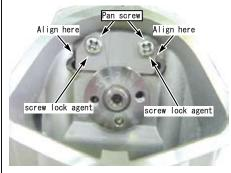
O Install the cam chain onto the cam sprocket.
