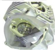
O Attach the cam stopper plate(kit included) to the SuperHead + R with apply lock agent to the pan screws(x2). At this time, align both ends of the cam stopper with the notches on the rocker arm shaft, attach them, and tighten them to the specified torque.
