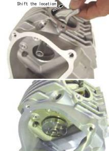
O Attach the cam stopper plate(kit included) to the SuperHead + R with apply lock agent to the pan screws(x2).
