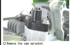
O Unfasten two screws holding the cam stopper plate on the cylinder head, and remove the cam stopper plate.
