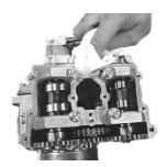
Insert the supplied 7x10 dowel pin to the dowel hole.
