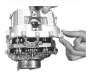
Remove camgear and both IN and EX camshaft.
