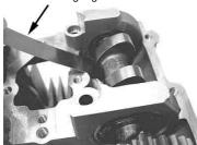
01-08-072 Install as stamped (IN, EX) of the camshaft.
