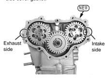
Attach the cylinder head left side cover to the cylinder head with nine 5x22 and two 5x15 socket cap screws. (See the foto below.) Lightly apply "Alumi Special", the heat-resistant lubricating agent , to the threaded portion of the screws.
