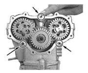
Lightly apply liquid gasket to the intake and exhaust sides of the cylinder head cover gasket which was attached to the mating surfaces of the cylinder head cover and cylinder head, and then install the cylinder head side cover gasket.
