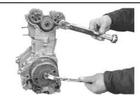
Attach the supplied 6x20 socket cap screw to the side of the cylinder head, and tighten it up. Degrease well the head-cover mounting surface of the cylinder head.
