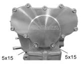
Tighten each socket cap screw diagonally in a few steps to the specified torque.
