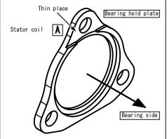
O Check the orientation of the bearing hold plate, and install the three 6x25 socket cap screws after applying thread locking agent.
