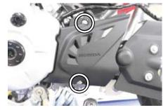
O Loosen and remove the bolts in several steps, and remove the L.crankcase cover. X Pull the L. crankcase cover by magnetic force. Do not get your fingers pinched as the tension is applied. Be careful.
