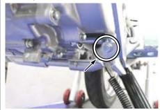
O Refer to the service manual and remove the bolts at the circled locations, then remove the left side body cover.
