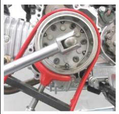
O Attach the spring washer and shaft nut included in the kit to the crankshaft.
