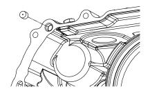
Attach R. Crankcase cover, clamp and cable receiver COMP. with genuine bolts, divide bolts several times diagonally and tighten to specified torque.
