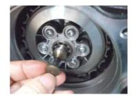
Attach the O-ring(120mm) to the clutch cover and apply a engine oil to the O-ring.
