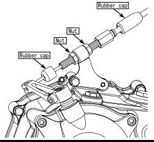
Clutch free play 10 to 20 mm at the clutch lever end
