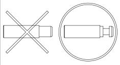
♠ Note: If use the oil hole plug (00-02-0111), the oil passage will be closed and the engine may be damaged.
