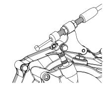
Turn the clutch release pinion clockwise until it stops, and insert a plain washer into the release pinion.
