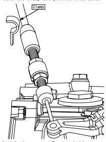
· Attach the removed R. step holder.
