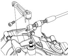
Adjust the clutch free play at the adjustment part of the clutch cable, tighten the nut to the specified torque, and cover each with a rubber cap.
