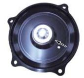
Attach the O-ring(120mm) to the clutch cover and apply a engine oil to the O-ring.
