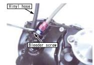
• Tighten the bleeder screw to the specified torque.
