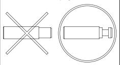
♠ Note: If use the oil hole plug (00-02-0111), the oil passage will be closed and the engine may be damaged. • When installing an oil hose to the oil outlet of the cylinder
