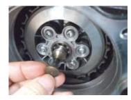
Attach the O-ring(120mm) to the clutch cover and apply a engine oil to the O-ring.
