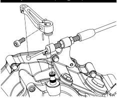
Adjust the clutch free play at the adjustment part of the clutch cable COMP. tighten the nut to the specified torque, and cover each with a rubber cap.
