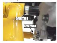
Attach R. step holder with shim ring (12x18x0.5), U nut (M12x1.25), washer (8mm) and hex bolt (8x45).
