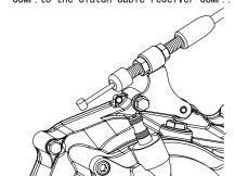
Turn the clutch release pinion clockwise until it stops, and insert a plain washer (10mm) into the clutch release pinion.
