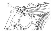
Attach R. Crankcase cover, clamp and clutch cable receiver COMP. with flange bolt(6x40), divide bolts several times diagonally and tighten to specified torque.
